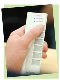
clearly understood. Students respond using a clicker, a handheld transmitter about the size of a TV remote. An infrared or radio-frequency signal beams the responses to a receiver attached to the instructor's computer, where
